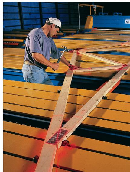
■ Laser projection reduces tooling set-up and truss assembly times.
