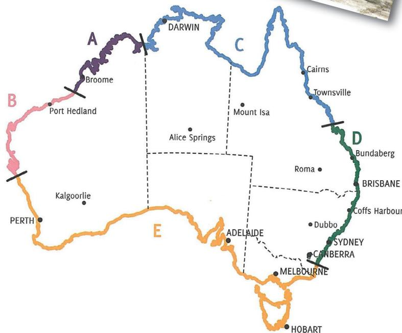
**Figure 8.4** COASTAL ZONES RELATED TO CORROSION DUE TO AIRBORNE SALT
