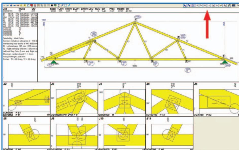
Figure 2: The MiTek JigCentre Paperless screen with Planx Link controls (top right) integrates seamlessly with Matchpoint Planx automated tooling.
