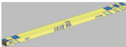
Figure 1: An example of assembly data extracted from design software and printed on a wall frame component.
