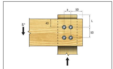
close to timber ends or edges have to be regarded as ineffective. Brackets must not be hung too low or too high such that their fasteners will be too close to timber edges.
