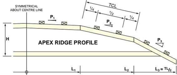
trusses without requiring the use of CAD. The appropriate set of formulae depends on whether there are odd (truncated ridge) or even (apex ridge) numbers of top chord segments.
