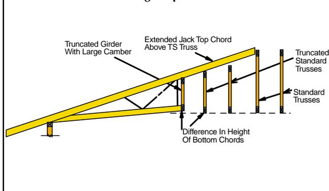
with tiles or sheet. In addition the height difference between bottom chords on the Truncated Girder and Truncated Standard may create difficulties for the plasterer.
