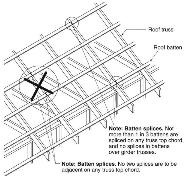
reported as "failed" only to find on inspection that the top chord has buckled - allowing the bottom chord to drop down. One of the common causes of buckling of girder top chords is the ineffective nailing of battens.
