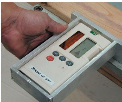
■ A laser camber measurement system will provide a fast way of measuring and setting camber.
