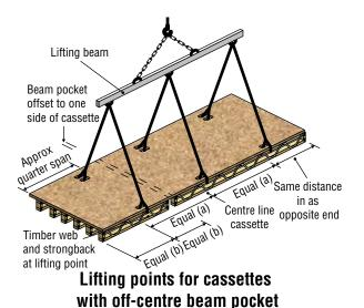
c. The above methods of lifting suit a crane on site, and an overhead gantry in the factory. Where a gantry is unavailable or cannot be used, a method of lifting and handling in a manufacturing plant has to be devised without distorting or damaging the completed cassette. A forklift accessory with multiple prongs described earlier is a suitable option for this purpose.
