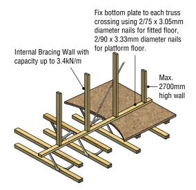
Braced walls perpendicular to trusses with bracing capability up to 3.4kN/m
