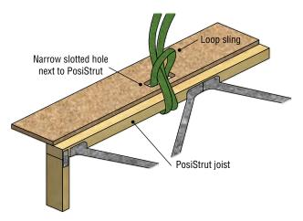
Where a sling is wrapped around the outer joist as shown, the recessed flooring edge should be located in the direction of laying the cassettes, so that the slings do not get trapped in between cassettes.
