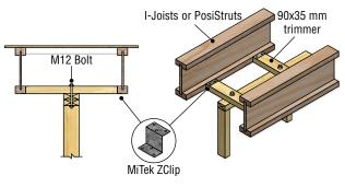
Z-Clip detail to transfer lateral forces to internal bracing walls
