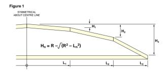
spacing. The total length (span plus overhangs) of the truss divided by the chosen total number of top chord segments should fall within this range.
