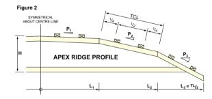
trusses without requiring the use of CAD. The appropriate set of formulae depends on whether there are odd (truncated ridge) or even (apex ridge) numbers of top chord segments.
