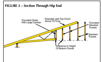
with tiles or sheet. In addition the height difference between bottom chords on the Truncated Girder and Truncated Standard may create difficulties for the plasterer.
