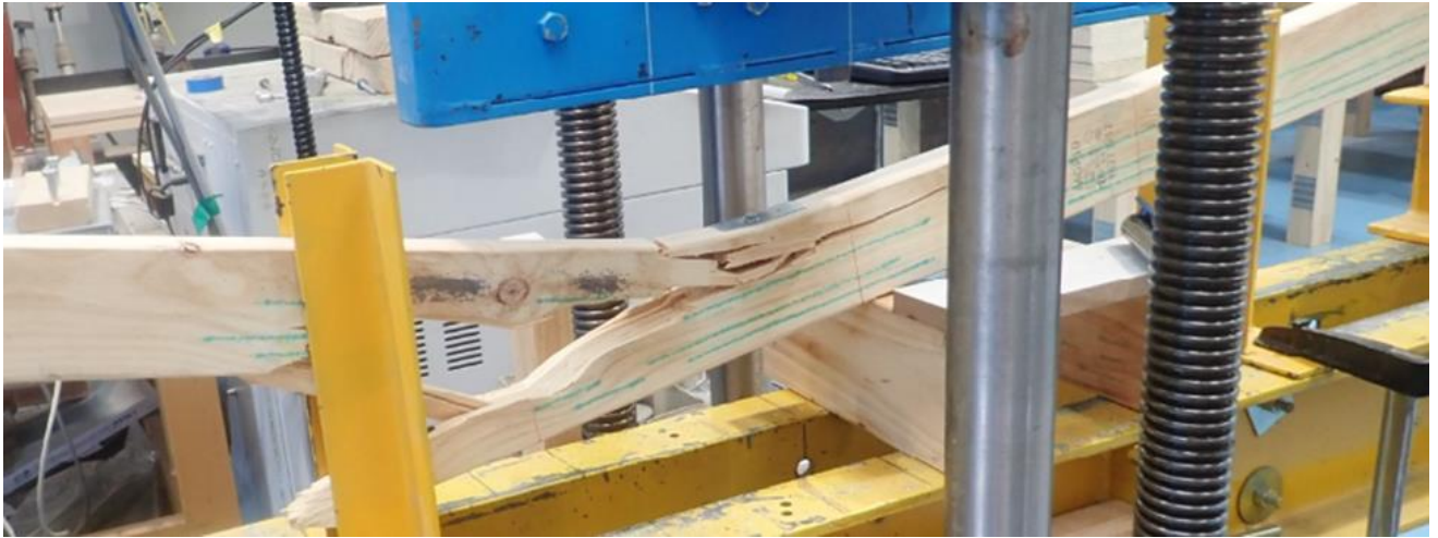
Figure 2: Typical bending fracture pattern of unmodified solid timber
