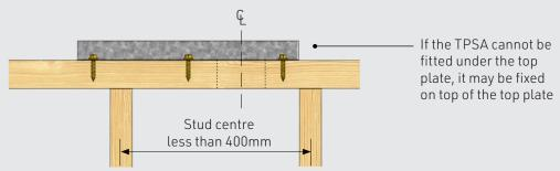
3. Fix 10 MiTek screws to the pattern shown in the drawings below.
