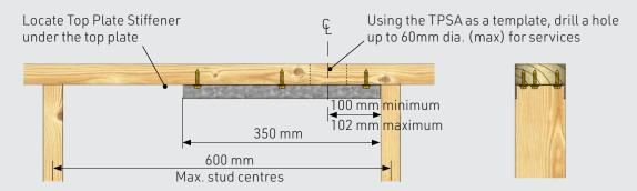
2. If the studs are too close together, and if there is no truss above, the TPSA may be installed on top of the top plate with no restrictions on the location of the 60mm dia. hole.
