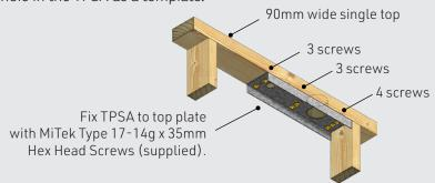
5. Any tiedown of a truss or framing timber from above may be fixed to the top and/or of the top plate only.
